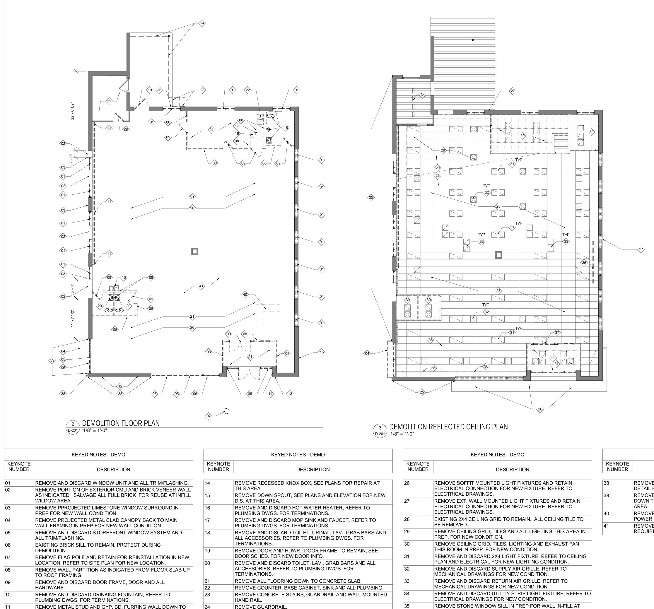
REMOVE METAL STUD AND GYP. BD. FURRING WALL DOWN TO CMU WALL. REMOVE ALL PIN MOUNTED SIGNAGE, SIGNAGE IS NOT 12 POWERED. REMOVE ADA POWERED DOOR SWITCH, SEE PLANS FOR REPAIR 13 AT THIS AREA.
