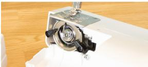
• Locate the bobbin case by removing the free arm. Pull down the bobbin case cover and remove the bobbin case.
