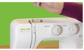
• Raise the presser foot. Turn the handwheel counter clockwise to bring the needle up to the highest position. Thread the take-up lever from right to left (step #3 on the machine). Finish threading through the needle bar thread guide.
