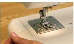
• Thread the needle from the front to back. Then, pull the loop through and your needle is threaded. Bring up the bobbin thread by holding the needle thread and turning the handwheel counterclockwise. The bobbin thread will loop around the needle thread. Pull the loop through to retrieve the bobbin thread.
