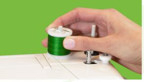
• Place the thread on the spool pin. Follow the numbered thread path shown on the machine.
